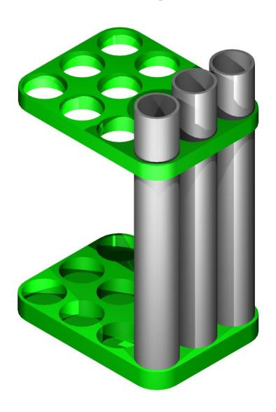
Continue to locate and twist the conduits into their locations, working your way around the complete storage unit.
