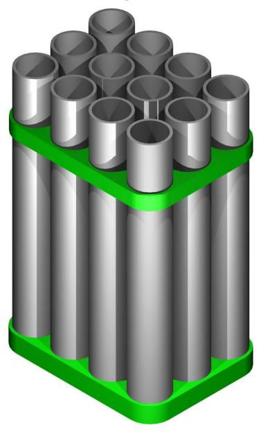
The 25 mm conduits simply serve as a holder to locate the small conduits, which store your items. Next we get to work on the 20 mm conduits.
