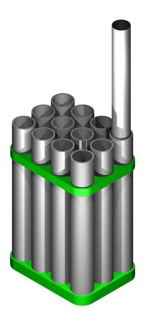
Place the 20 mm conduit with the plug in place. (BTW the plug is simply there to stop stuff falling out), and as the plug is located into the next conduit, place the drying conduit in place, do not allow the glue to leak to the outside of the small conduit as it might contact the outer conduit and stick to it, restricting it's removal, Use the glue sparingly. The preference would be for a gel type supa glue.
