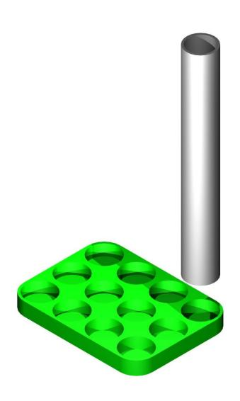
After deburring the base section, and lightly sanding the conduit, locate the conduit into the base by twisting, and pushing at the same time. The conduit needs to be tight but not to tight as to damage the base.
