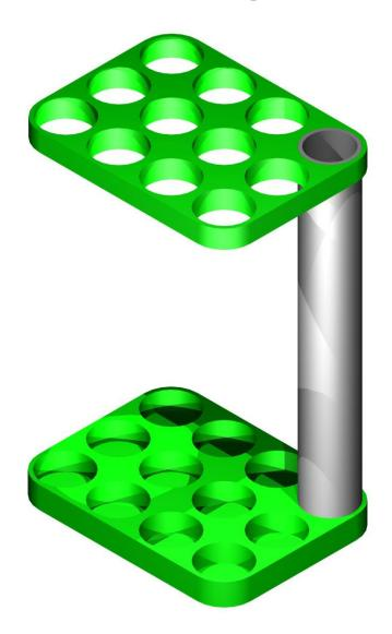
Locate the top section on the conduit after deburring the bottom of the part, and ensure that the fitment is tight but not too tight as to damage the part.
