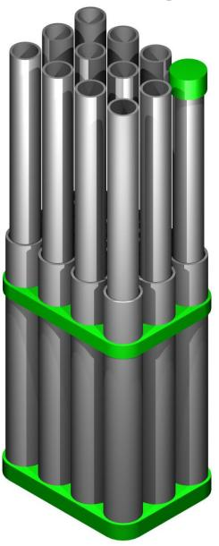
When placing the cap onto the 20 mm conduit, it needs to be firm but not too firm to remove. The shape edge does need to be sanded down so as not to leave a cutting edge, but just a raised smooth ridge to aid in removing the cap. To obtain this firm but not too firm fitment, the conduit may also need to sanded slightly, but only ever so slightly, as you do not want the caps to fall off, if the unit falls over. After all that is the reason for the caps, so that you don't loose stuff.
