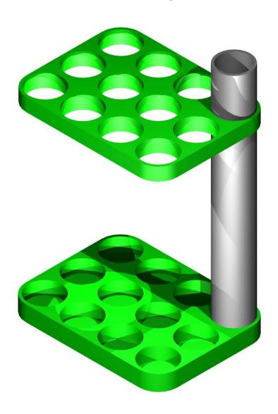
Measure down 30 mm and this will be the final location for the top section. This will depend on you and where you want the top section to be located. I place the test shots in about this location and they seemed to work rather well, providing a balanced storage unit.
