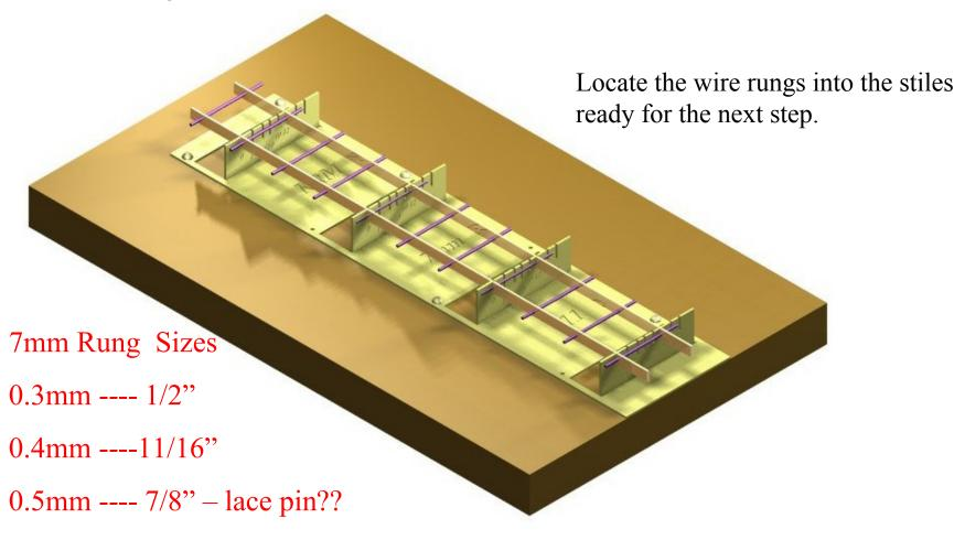
To make the ladder stiles (the ladder) square, push the stiles and rungs hard up against one of the vertical sectors. You can now solder the rungs that are NOT near the sectors, on one side. Check the ladder for square again then solder the other side of the same rungs in place. Please use the solder sparingly as an excess build up of solder will look
