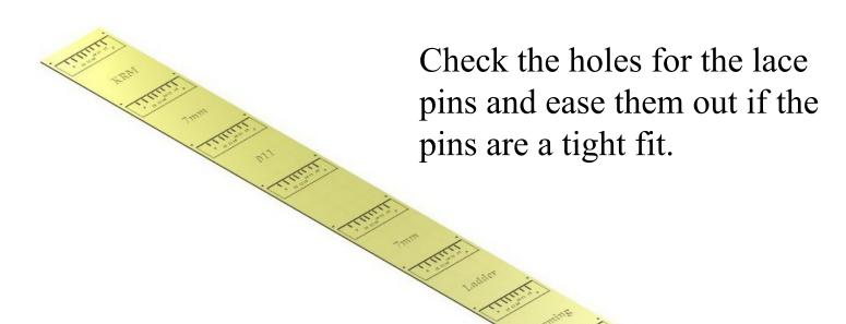
Try not to bend or warp the etch when handling it, as it easier to work with if it is flat.
