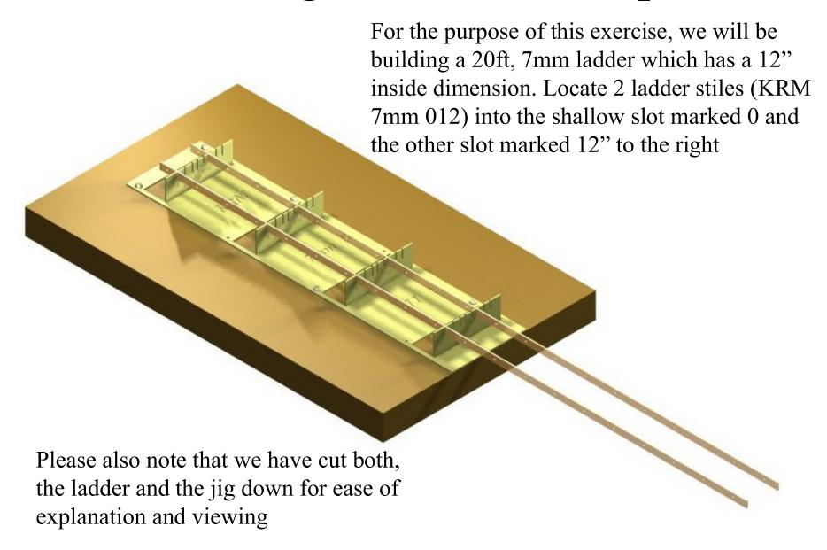
The stiles can be drilled out to suite, they are etched at approx 0.35mm. The ladder rung is very simply your choice. Ensure that when drilling the stiles, take care not to bend or warp them. You can also use small sections of masking tape to hold the ladders stiles in place whilst working on them.
