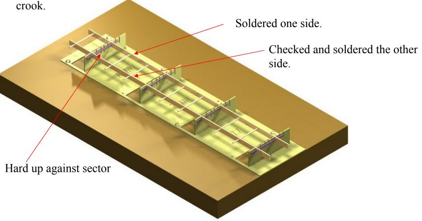
Move the ladder in the jig so that the unsoldered rungs can now be soldered in place.
