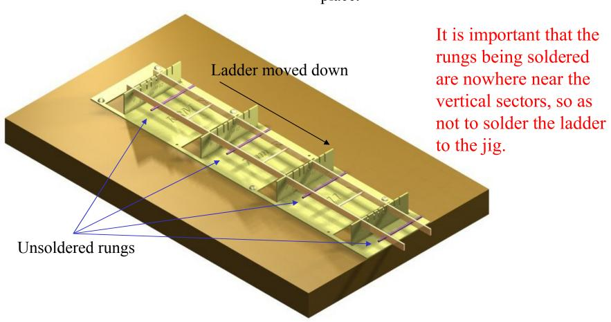
Remove the newly formed ladder from the jig. Trim the excess rung material on the outer side of the stiles with a sharp pair of cutters.
