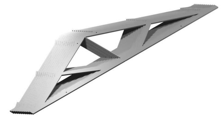
The truss jig consists of 5 pieces of 3 mm acrylic.
